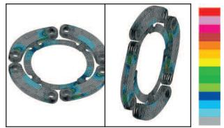
Using finite element analysis (FEA), the disc design can be easily modified along with changes in the composite material. Custom disc designs (manufactured on state-ofthe-art laser cutting machines) can add to or lessen coupling flexibility or increase strength and stiffness as required for the particular application. There are over
