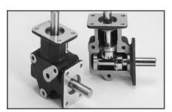
Crown Right Angle Gear Drives Two and three way models with 1:1 and 2:1 ratios. Spiral bevel gears. 3/8 to 1 inch dia. Stainless steel shafts.
