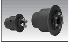
H-TLC Torque Limiters Corrosion proof design. Adjustable. Bores from .250" to 1.000". Torques from 4 to 500 in. lbs.
