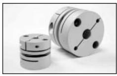
ServoClass<sup>®</sup> Single Disc Couplings Zero backlash, smaller package with higher torsional and axial stiffness. Clamp hubs. 8 sizes. Torques to 880 in-lb. Inch and metric bore.
