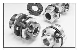
**CD® Couplings** Composite disc design that outperforms steel discs and elastomeric models. Torsional stiffness. 3° misalignment. Torques to 500,000 in. lbs.
