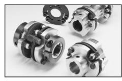
**CD® Couplings** Composite disc design that outperforms steel discs and elastomeric models. Torsional stiffness. 3° misalignment. Torques to 500,000 in. lbs.
