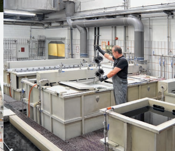
Manuell bediente Eloxalanlage Manually operated anodizing plant
