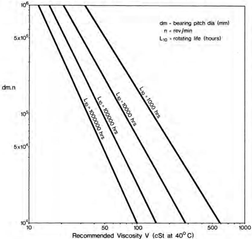
This graph is valid for normal ambient temperature conditions and where there is reasonable heat dissipation.
