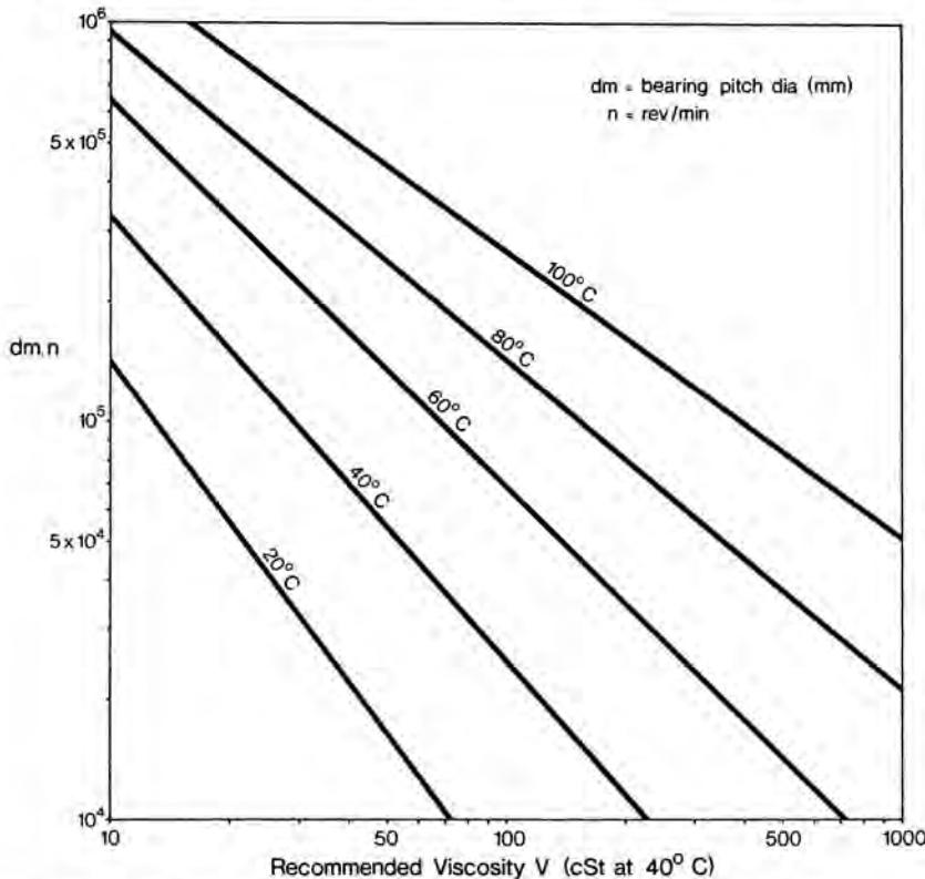
The temperature relates to the actual temperature that the bearing achieves, or is estimated to achieve, in service when taking into account all environmental and operating conditions.
