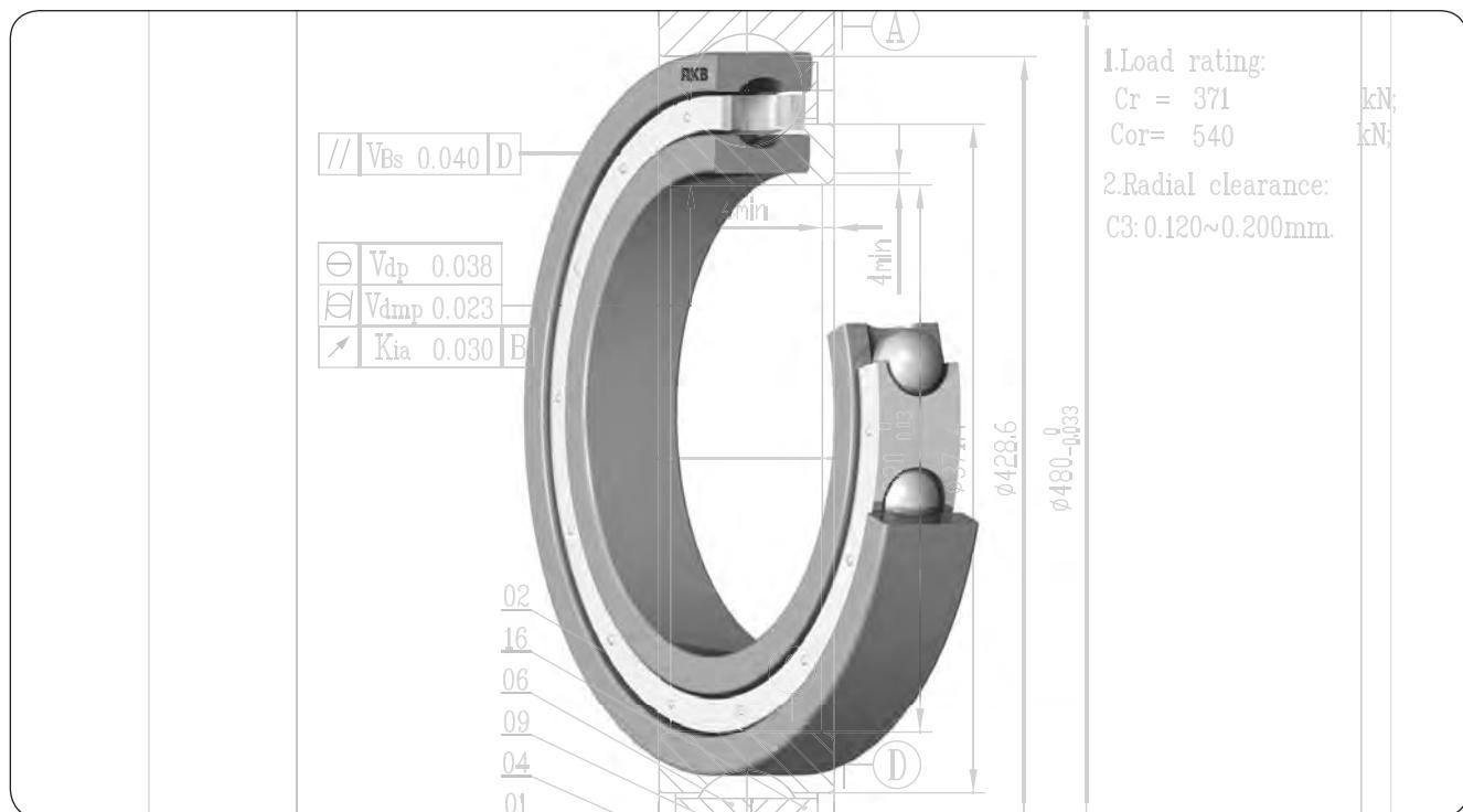
The axial clearance is generally not standardized and depends on the values of the radial clearance, ball size and raceway radius.
