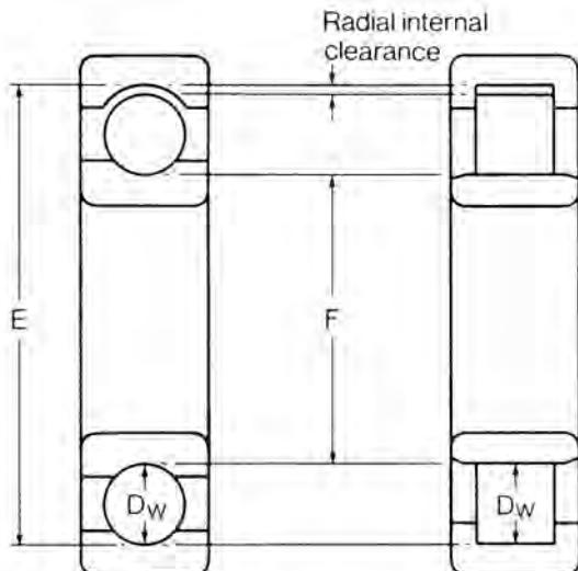
Bearing radial internal clearance relates to the total clearance between the raceways and rolling elements measured normal to the bearing axis.
