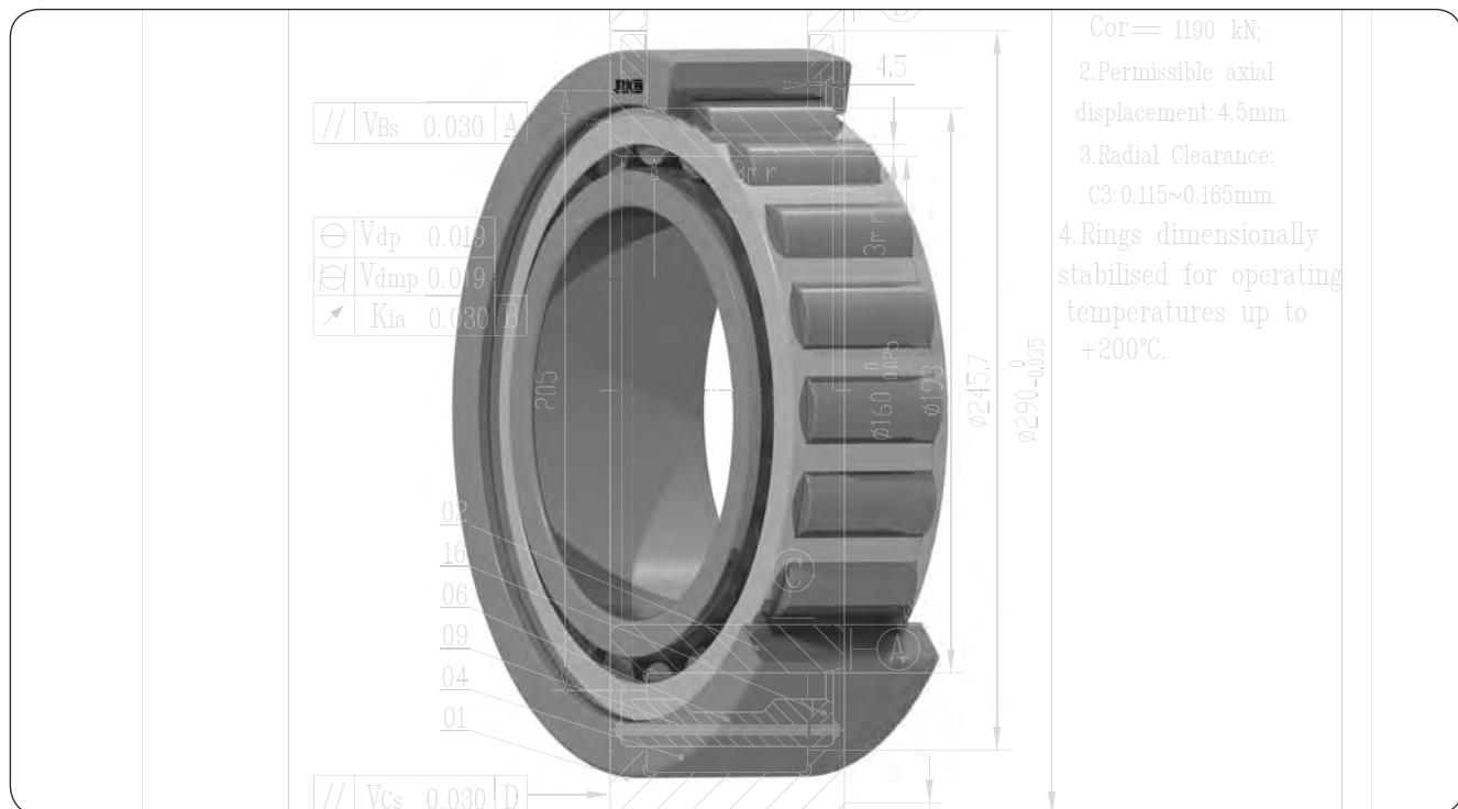
Depending on size and design, the bearings are equipped as standard with one of the following cages: unhardened pressed steel roller centered, one-piece window type brass inner or outer ring centered, two-piece machined brass roller centered (suffix M) or outer ring centered (suffix MA) or inner ring centered (suffix MB) and steel pin-type for pierced rollers.
