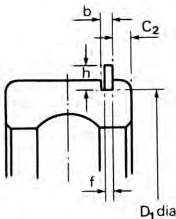
**Snap ring and groove tolerances – metric bearings
