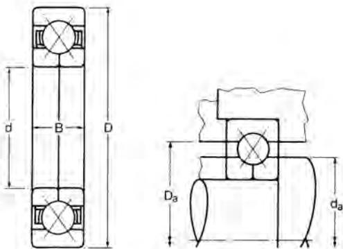
Duplex bearings are also available in the model series Q2 with split outer ring with same data.
