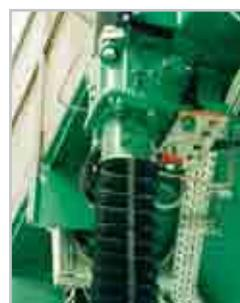
Installation of lifting system with bellows-type casing for approx. 9 m of lift.
