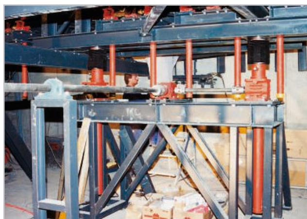
High-performance spindle lifting systems compliant with VBG 70 for adjusting the height of hall platforms
