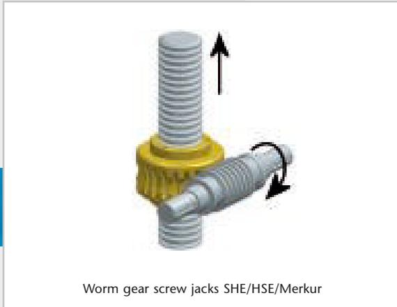
Drive is provided by the worm-drive shaft acting on the worm gear with female thread. Lifting movement is provided by the spindle anti-turn device (supplied with unit or added onsite).
