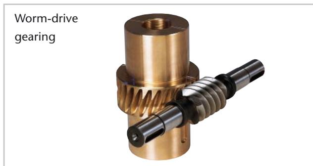
The tooth profile play (when new) of 0.1 – 0.3 mm varies, according to the size of the unit or amount of axle clearance, with the rate of wear
