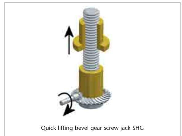
Drive is provided by the driving pinion acting on the bevel gear. Rotating movement is provided by the positive engagement of the spindle in the bevel gear. Lifting movement is provided by the traveling nut anti-turn device fitted onsite. The alignment of the bevel gear (Ro = wheel up / Ru = wheel down) determines the direction of rotation (see type 1).
